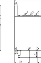
G = Gas Inlet 1/2" BSP Female W = Water Inlet 1/2" BSP Male D = Drain Outlet 1-1/4" BSP Male
